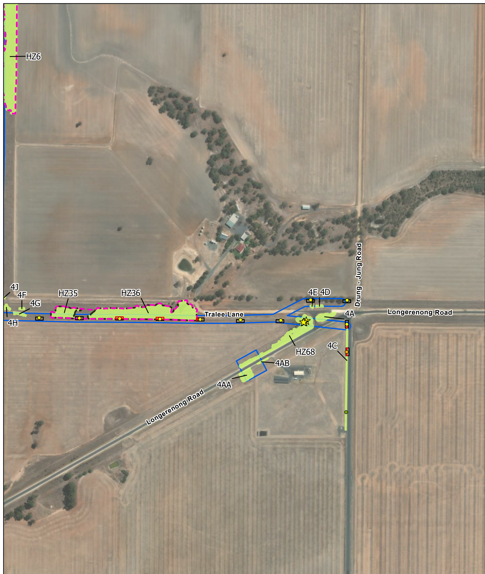
Figure 2-9: Native vegetation to be removed
